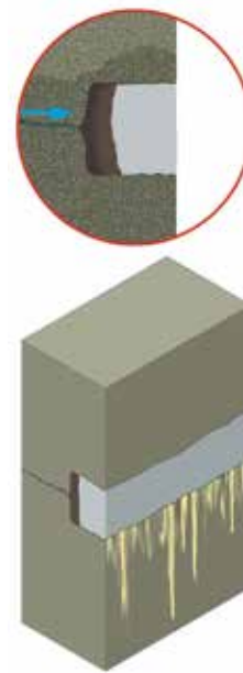
Step 3: Install Krystol Repair Grout.
