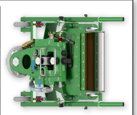
THE BASE FRAME LOCKING FUNCTION MAKES INSERTION OF THE LINER INTO THE INNER CHAMBERS EASIER.
