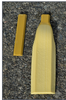
Before and after water exposure
