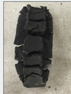
Bentonite waterstops can disintegrate over time while Krytonite will continue to stop water.
