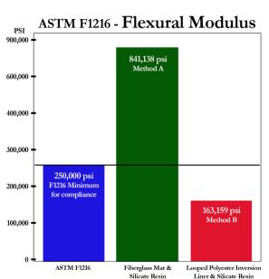
\* ASTM (American Society for Testing and Materials) F1216 - Standard Practice for Rehabilitation of Existing Pipelines and Conduits by the Inversion and Curing of a Resin-Impregnated Tube.
